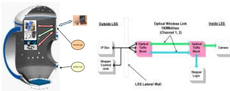
*Advantage: Non-intrusive, optical data connections experiment*
