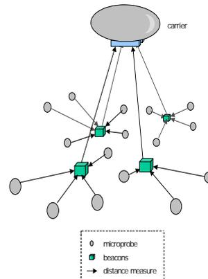
*Advantage: Sensors Localisation utilizing RF wireless, very low mass and power*
